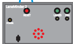
LaneMinder2 Lane intrusion warning system - not connected to MachineMinder safety system
