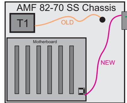
Locate the wire that goes from the T1 secondary to C2A-22j and remove it from the C2A block. Cut off the connector and insulate the end of the wire (take care as it will still be live with 90VAC).
