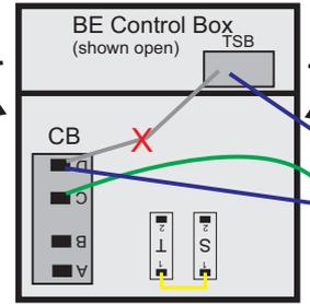
Remove both ends of the wire connected between CB terminal D and TSB.
